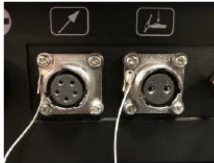
Remote sockets wiring configuration
