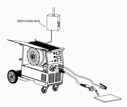
Insert the quick plug of the gas / no gas selector into the "-" output terminal on the middle plate of the welding machine, and tighten it clockwise.
