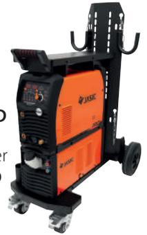
The Jasic TIG 315 is a digital AC/DC inverter welder with a wide range of functions, high performance and advanced technology. This multi-function welder with AC TIG welding (square wave, triangular wave and sine wave), AC pulsed TIG welding, DC TIG welding, DC pulsed TIG welding, AC-DC hybrid TIG welding and coated electrode MMA welding (DC, AC).
